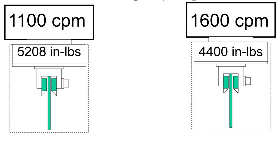
$\frac{5208 \times 0.0142 \times 1100 \times 1100}{1,000,000} = 89 \text{ tons} \quad 159.94 = \frac{4400 \times 0.0142 \times 1600 \times 1600}{1,000,000}$
