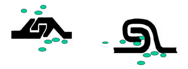
Hot rolled sheets have tighter tolerances that keep larger particles out. Large particles cause hitch hiking of the sheets. Hitch hiking
