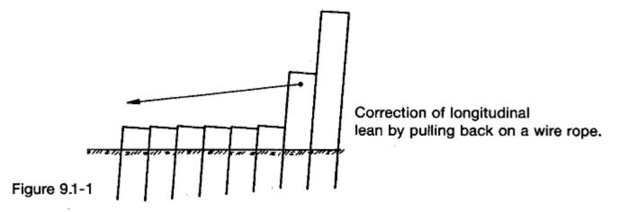
In conjunction with the above method, the hammer can be placed off centre of the pair of piles towards the last driven piles.
