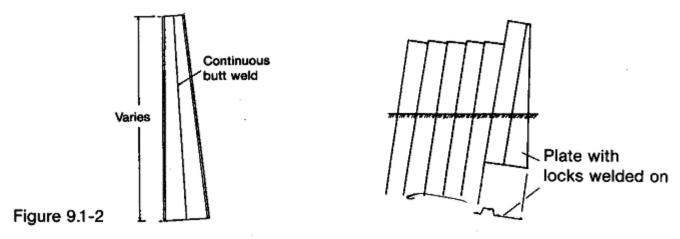
When, in spite of all precautions, a lean cannot be eliminated, taper piles must be employed to correct the error. Copyright © 2016 American Piledriving Equipment Inc. All Rights Reserved
