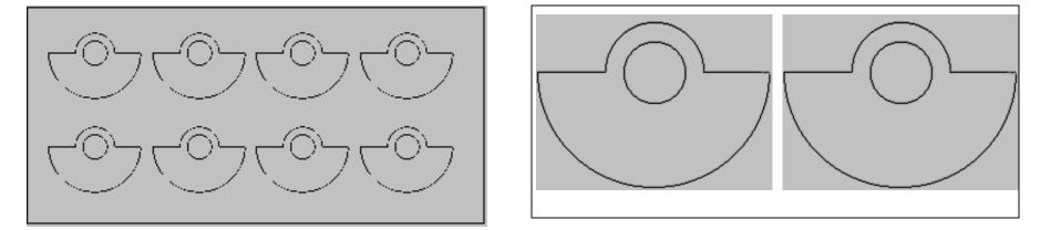
More vibrating weight Less amplitude Less vibrating weight More amplitude
