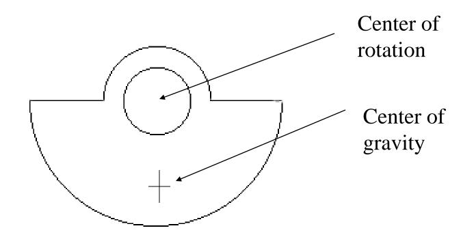
Eccentric moment = distance between the center of rotation and the center of gravity  $\mathbf{x}$  the total mass of the eccentric.
